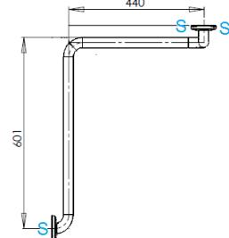
It is recommended to set up the horizontal part of the bar between 700 and 750 mm height, with respect to the ground.
